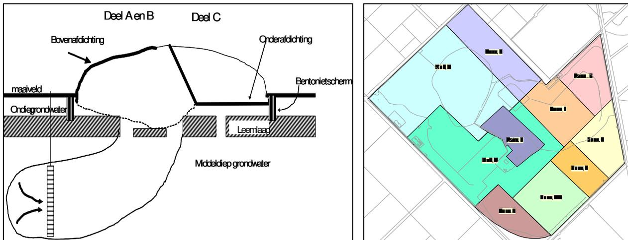
Figure 1. Cross-section and plan of the Vlagheide landfill
